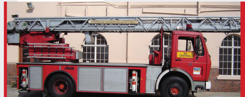
The old Metz Turn Table Ladder based on a 1981 Mercedes Benz 1419 chassis
