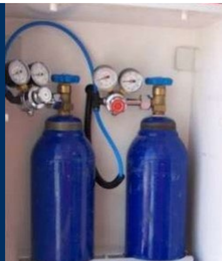
Oxygen cylinders are arguably one of the greatest risks to safety in the rear of an emergency vehicle
